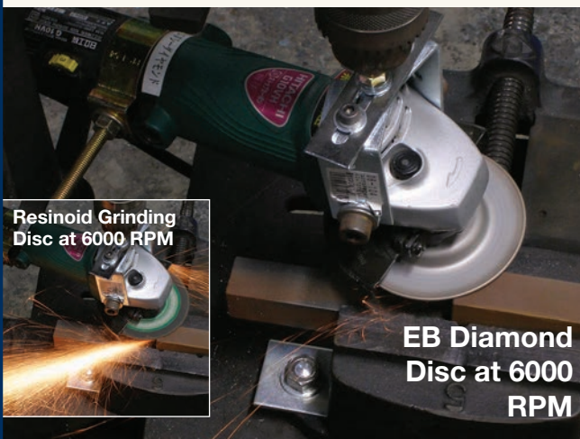
EB diamond grinding discs reduce sparking up to 1/100 of that produced by resinoid grinding wheels (inset left).
