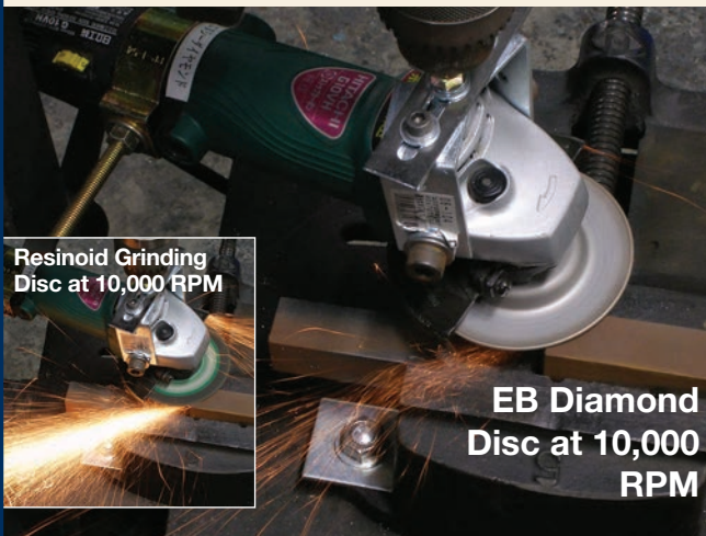
EB diamond grinding discs reduce sparking up to 1/100 of that produced by resinoid grinding wheels (inset left).
